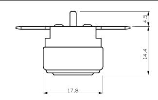
Description: Thermostat with bimetal snap-action disc and manual reset in ceramic housing.
